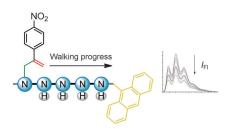
Charge of the light brigade: A molecule is able to walk back and forth upon a five-foothold pentaethylenimine track without external intervention. The 1D random walk is highly processive (mean step number 530) and exchange takes place between adjacent amine groups in a stepwise fashion. The walker performs a simple task whilst walking: quenching of the fluorescence of an anthracene group sited at one end of the track.
