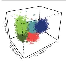
Better safe than sorry: A combined analytical procedure consisting of Raman spectroscopy and chemometrics can be used to test for anthrax endospores in environmental samples. Time-consuming enrichment steps are not required and low levels of anthrax endospores in household substances like baking powder can be detected within 3 h and discriminated against other nonpathogenic Bacillus species with typing accuracies of up to 99%.
