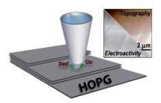
After all, it's active: High-resolution scanning electrochemical cell microscopy (SECCM) demonstrates that electron transfer at the basal plane of highly oriented pyrolytic graphite (HOPG) is fast. This finding requires radical revision of the current textbook model for HOPG electrochemistry.
